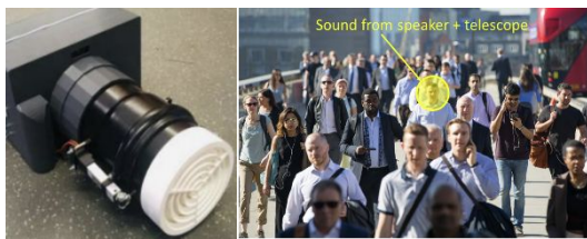
Figure 1. (a) Photograph of acoustic telescope with auto-zoom lens, designed to deliver sound to a target listener. (b) A potential application, connecting acoustically with a single person in a crowd [1].
