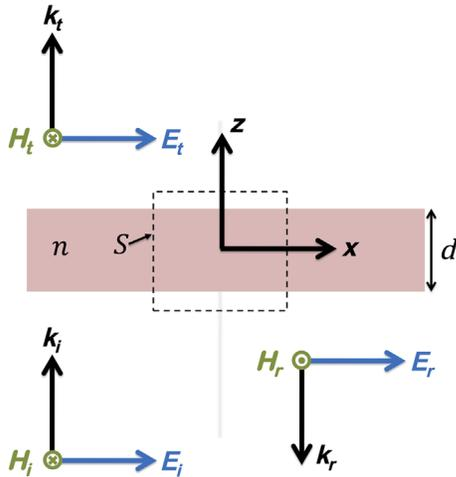
FIG. 7. Schematic view of a dielectric slab of thickness  $d$  with refractive index  $n$  illuminated with a linearly polarized plane wave. The reflected and transmitted electric and magnetic fields are depicted. The dashed box shows the closed surface for integrating the Maxwell stress tensor.
