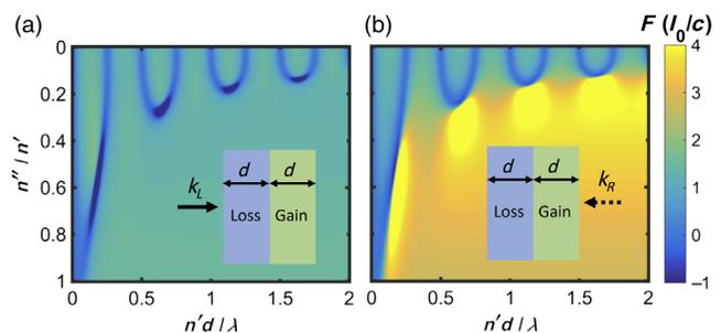
FIG. 3. Optical force exerted on a one-dimensional  $\mathcal{PT}$ -symmetric structure. (a),(b) Normalized optical force exerted on a bilayer made of balanced gain and loss as a function of the refractive-index ratio, i.e.,  $(n''/n')$ , and thickness of the dielectric layers for forward ( $k_L$ ) and backward ( $k_R$ ) plane-wave illuminations, respectively. The yellow and blue (in the color bar) correspond to the pushing and pulling forces, respectively.
