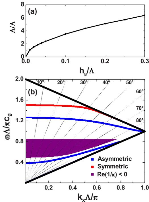
FIG. 4. (Color online) (a) Dependence of the wavelength width of the attenuation band,  $\Delta$ , with the gap thickness,  $h_g$ , for normal incidence. (b) Dispersion with respect to the parallel momentum of the even and odd modes and the region of negative  $\text{Re}(1/\kappa)$ . The geometrical parameters are:  $a=\Lambda/3.75$ ,  $h_m=\Lambda/1.875$ , and  $h_g=\Lambda/10$ , as in Fig. 3(c). Dotted lines show the dispersion of incoming plane waves for different angles of incidence.
