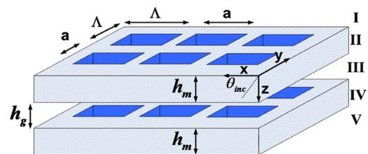
FIG. 1. (Color online) Schematic of an ADF metamaterial. The metal plates of thickness  $h_m$  and gap separation  $h_g$  are perforated with square holes of side  $a$  in a square lattice of period  $\Lambda$ .  $\theta_{inc}$  defines the angle of incidence with respect to the normal.
