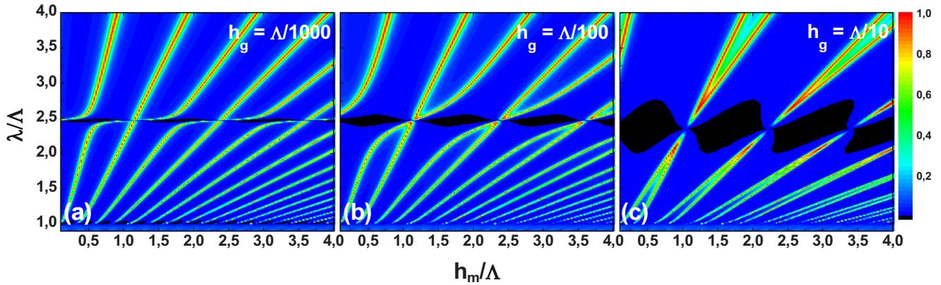
FIG. 2. (Color online) Normalized-to-unit-cell transmittance spectra as a function of  $\lambda$  and  $h_m$ , both in units of  $\Lambda$ . In the three panels,  $a=\Lambda/3.75$  and three different values of  $h_g$  are studied:  $h_g=\Lambda/1000$ ,  $\Lambda/100$ , and  $\Lambda/10$ . The incident sound plane wave is impinging at the normal direction.
