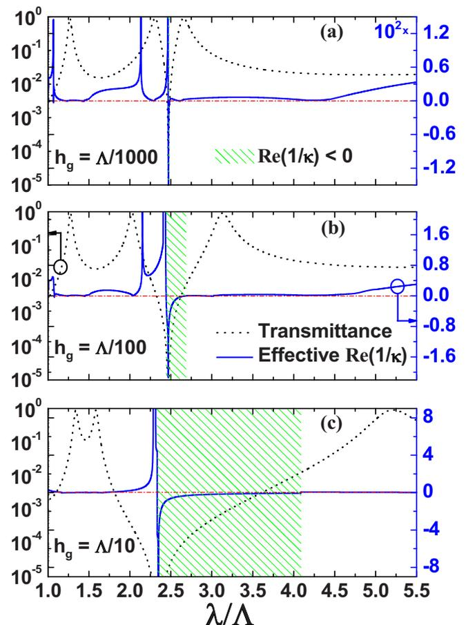
FIG. 3. (Color online) Normalized-to-unit-cell transmittance for normal incidence in logarithmic scale and the real part of the effective bulk modulus,  $\text{Re}(1/\kappa)$ , for ADF structures of square holes  $a=\Lambda/3.75$  and gap separations  $h_g=\Lambda/1000$ ,  $\Lambda/100$ , and  $\Lambda/10$ , respectively. In the three cases, the thickness of the plates is fixed at  $h_m=\Lambda/1.875$ . The shaded area highlights the area of negative  $\text{Re}(1/\kappa)$ .
