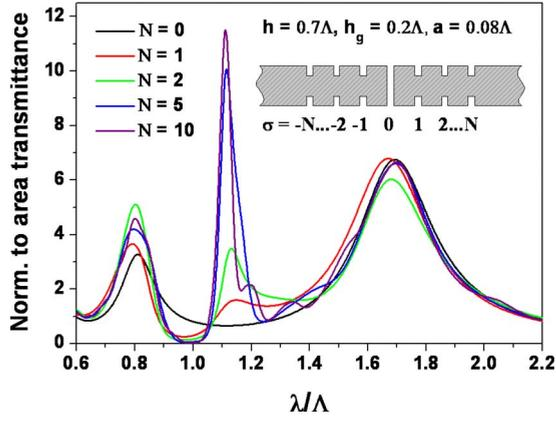
FIG. 2. (Color online) Influence on the normalized to area transmittance spectra, dependent on the numbers of surface corrugations ( $N$ , see color legend for the value) with the geometries as specified in this figure. The acoustic plane wave is impinging normal incident on the structured system. The corrugations are symmetrically placed at the upper and lower side of the structure as the inset depicts.
