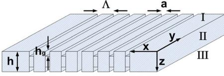
FIG. 1. (Color online) Schematics of a single slit surrounded by finite corrugations, made out of a perfect rigid body, impenetrable for airborne sound waves impinging on the structure.
